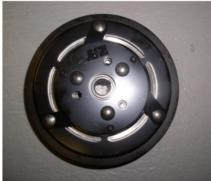
7. Install a 5/8-11-bolt (supplied) into the large threaded hole in the center of the clutch plate. Turn the bolt clockwise until the clutch plate dislodges, and remove.
