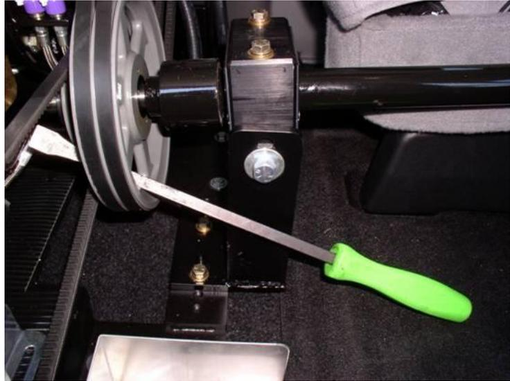
6. Remove the front clutch plate center bolt (1 1/4 x 5/16 - 24nf) that attaches the front portion of the two (2) piece clutch (see right).
