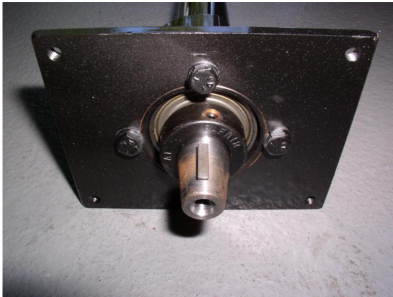
*NOTE: If you detect grease leaking from the Driveshaft, feel any excessive roughness or grinding, or there are signs that the Driveshaft got abnormally hot, the Driveshaft must be replaced.*
